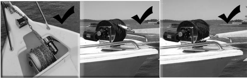
Rope direction can be either at upper or lower side of the drum
